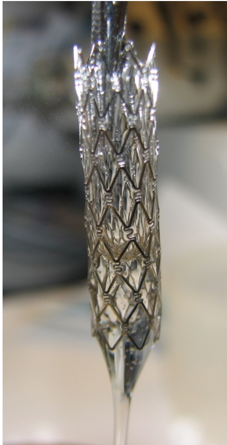
Figure 4.1: Removing excess PVA solution from stent after dip-coating. Gravity causes PVA solution to flow out of the stent – leaving behind a thin covering.
